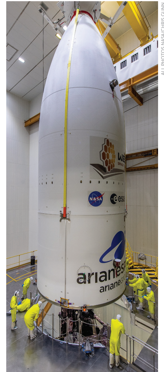
Encapsulated in its rocket fairing (protective cone) Ariane 5
